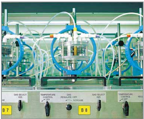
Static load method : proof ring type
