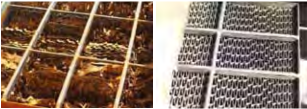
Regular steel used (serious corrosion shown)
