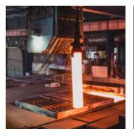
**Preheating** The process starts with reheating the bloom or ingot in our eight oxy-fuel heated pit furnaces.
