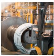
Preparation for cold drawing Rod coils are moved from the pre-dipping station to the cold drawing line.
