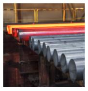
**Cooling** Bars are moved to a cooling bed before finishing operations.
