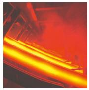
**Billet feedstock** Our rolling mill uses billet feedstock produced at the SMACC melting shop.
